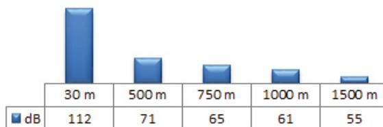
Reach of the sound at a medium noise level (70 dB) in a city, at all-round arrangement of the loudspeakers (180°)
